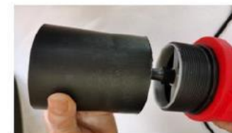
2. Installation of nozzle shields
