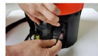
4. Connection of the power plug for the air gun to the power outlet for the aerosol sprayer
